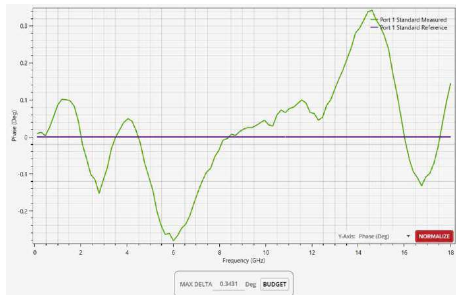
Figure 1. Normalized phase response between user-measured and factory-measured standard
