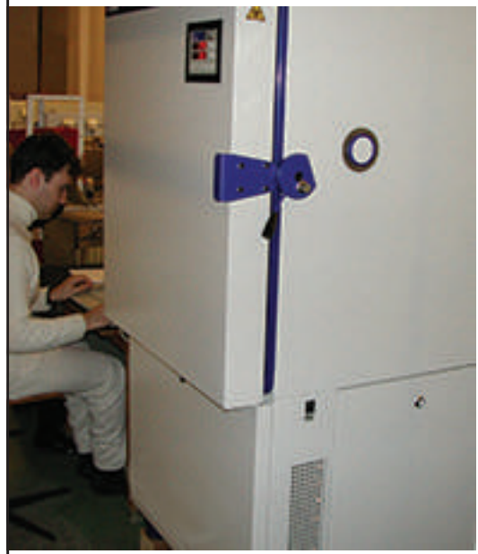
Temperature Chambers operating in the temperature range of -72°C to +200°C and Vacuum Chambers up to 150°C.
