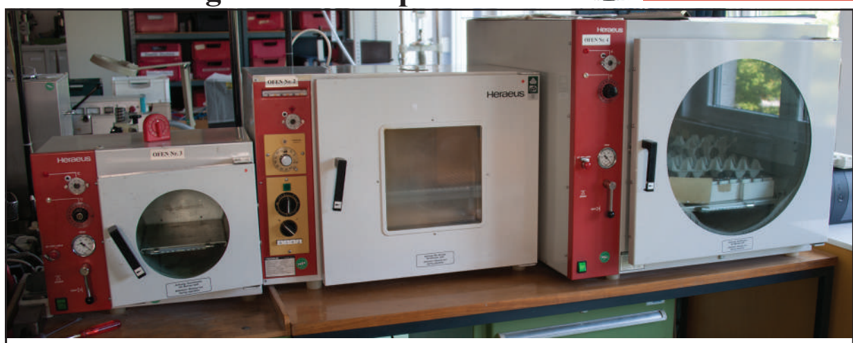
Temperature Chambers operating in the temperature range of -72°C to +200°C and Vacuum Chambers up to 150°C.
