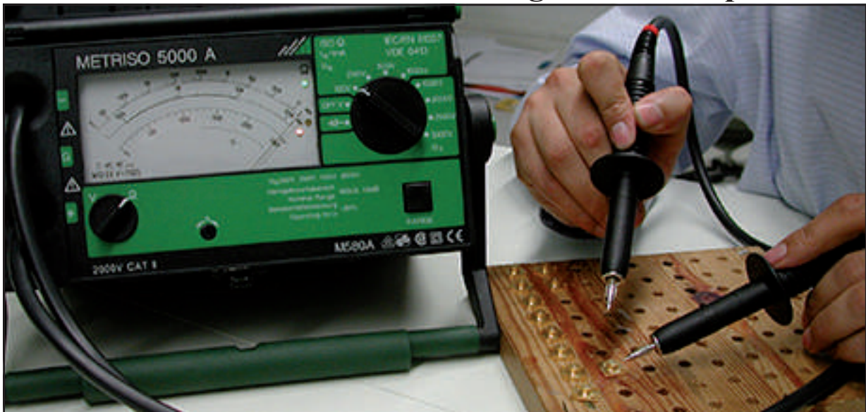
Insulation Resistance Test
