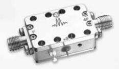
Marki Microwave offers a complete line of doublers, triplers, and quadruplers. All multipliers are constructed using silicon Schottky diodes, resulting in intrinsically lower phase noise performance compared to noisy GaAs devices. Our doublers and quadruplers are built using highly symmetric, monolithic diode bridge quads which provide cutting edge performance in terms of broadband coverage (as much as 25:1 bandwidth ratios) and superior fundamental suppression.
